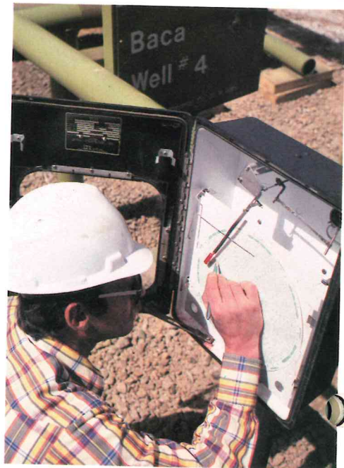
A Union Oil Company production foreman checks pressure readout on geothermal well in New Mexico.
