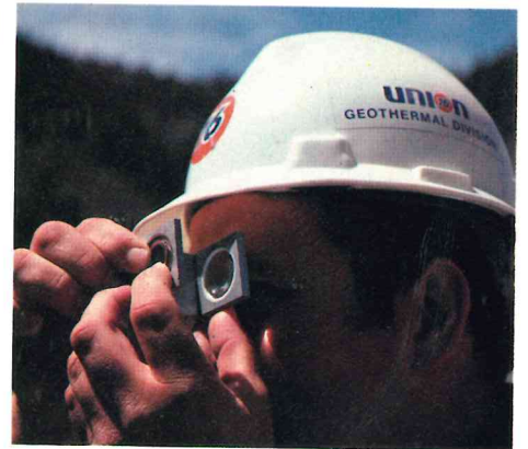
Left, specially-equipped rotary drilling rigs such as this one in New Mexico are used to drill geothermal wells. Top, well cuttings brought to the surface by circulating fluids tell a geologist the types of formations which the drill bit is penetrating. Above, drilling foreman "reads" film which measures the deviation of the well bore from vertical.
