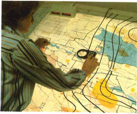
Left, computer plotting of a contour map of an area aids in determining the boundaries of a geothermal reservoir and selection of drilling locations.
